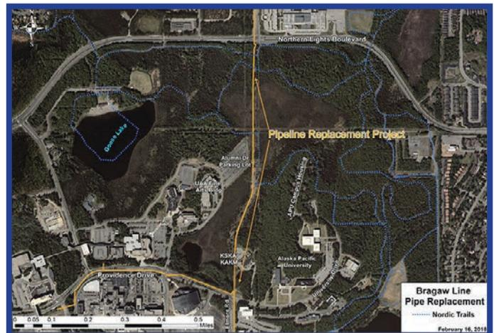
**What are you doing and why?** This project replaces 3,000 feet of 12" high pressure pipeline that was originally installed in the 1960s. The Bragaw Pipeline is critical to natural gas delivery in the Anchorage area. Replacing this segment of pipe will improve the safety and reliability of ENSTAR's system.
