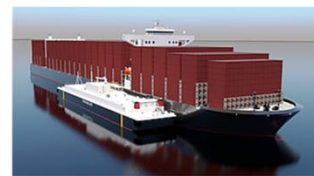
LNG Bunker Barge up to 416 feet smaller vessels are barges towed by tugs
