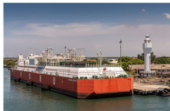
Floating storage plus onboard regasification smaller vessels are barges towed by tugs
